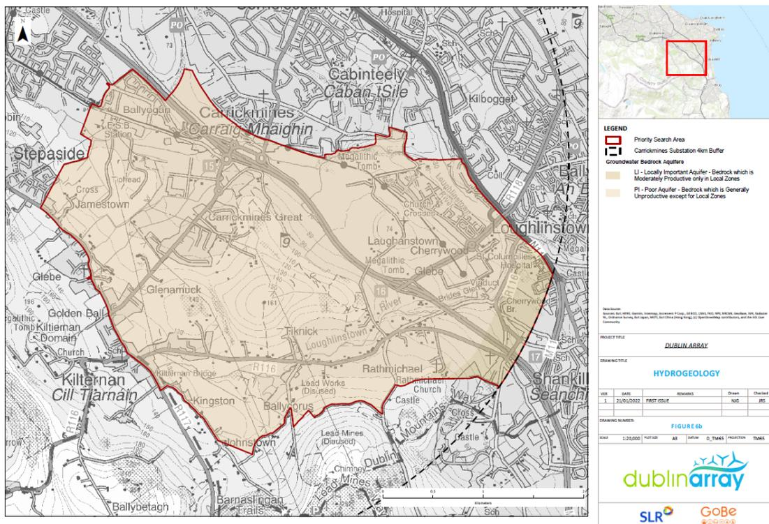
Figure 4.12 Groundwater Bedrock Aquifers
